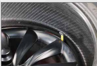
The mounting phase of the second bead is completed with the **simultaneous use of the bead breaker disc**, the rotation of the turntable and **in the presence of lowered tyres or RFT** with the use of the Press Mate which ensures that the tyre remains in the rim channel.
